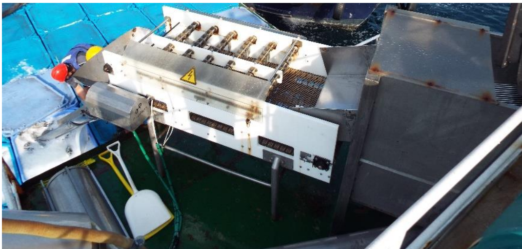
Figure 3. The stunning machine used by SÜRSAN to stun sea bass and sea bream. On the right of the photo is the dewatering unit.
