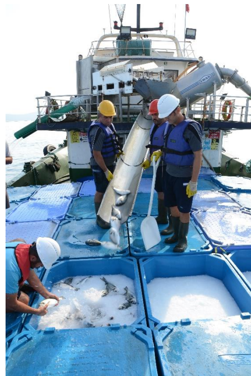
Figure 4. After electrical stunning fish are immediately directed into totes of ice slurry for chilling.
